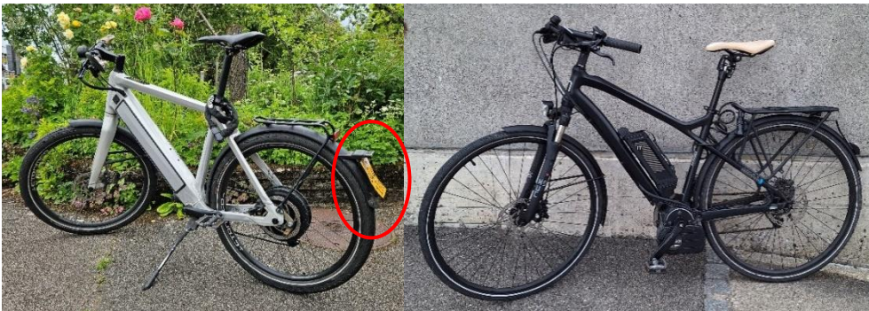
Fig. 9 Fast e-bikes (left) and slow e-bikes (right) can often only be distinguished by the yellow plate that is compulsory for fast e-bikes. Source: bfm.
