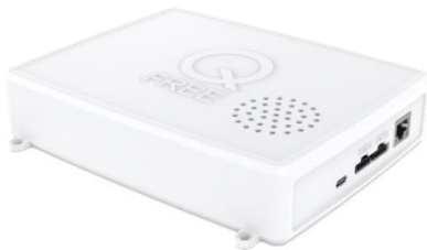
Fig. 3 Example of C-ITS “On Board Unit” (OBU) enabling ITS services on the vehicle side [19].
