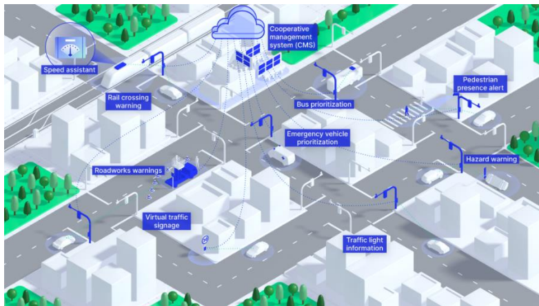
Fig. 51 Illustration of a CMS or Traffic Management Control in a C-ITS environment
