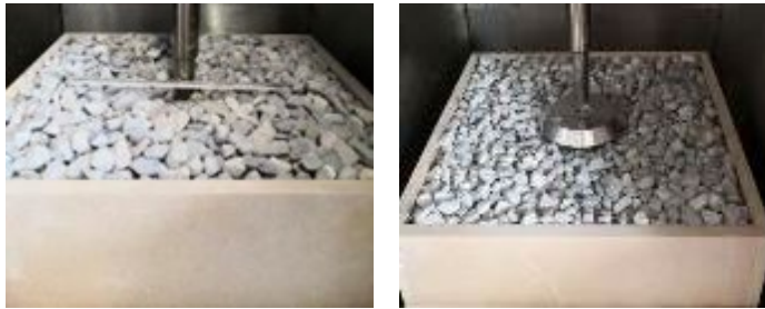
Abb. 24 photographs of the test specimens described in Abb. 23 at the end of the testing process (after several thousand of loading cycles). In the unreinforced specimens (left), the piston ended up deeply buried into the aggregate packing, while in the reinforced specimens (right), the piston with the loading plate is still visible at the surface of the aggregate packing.
