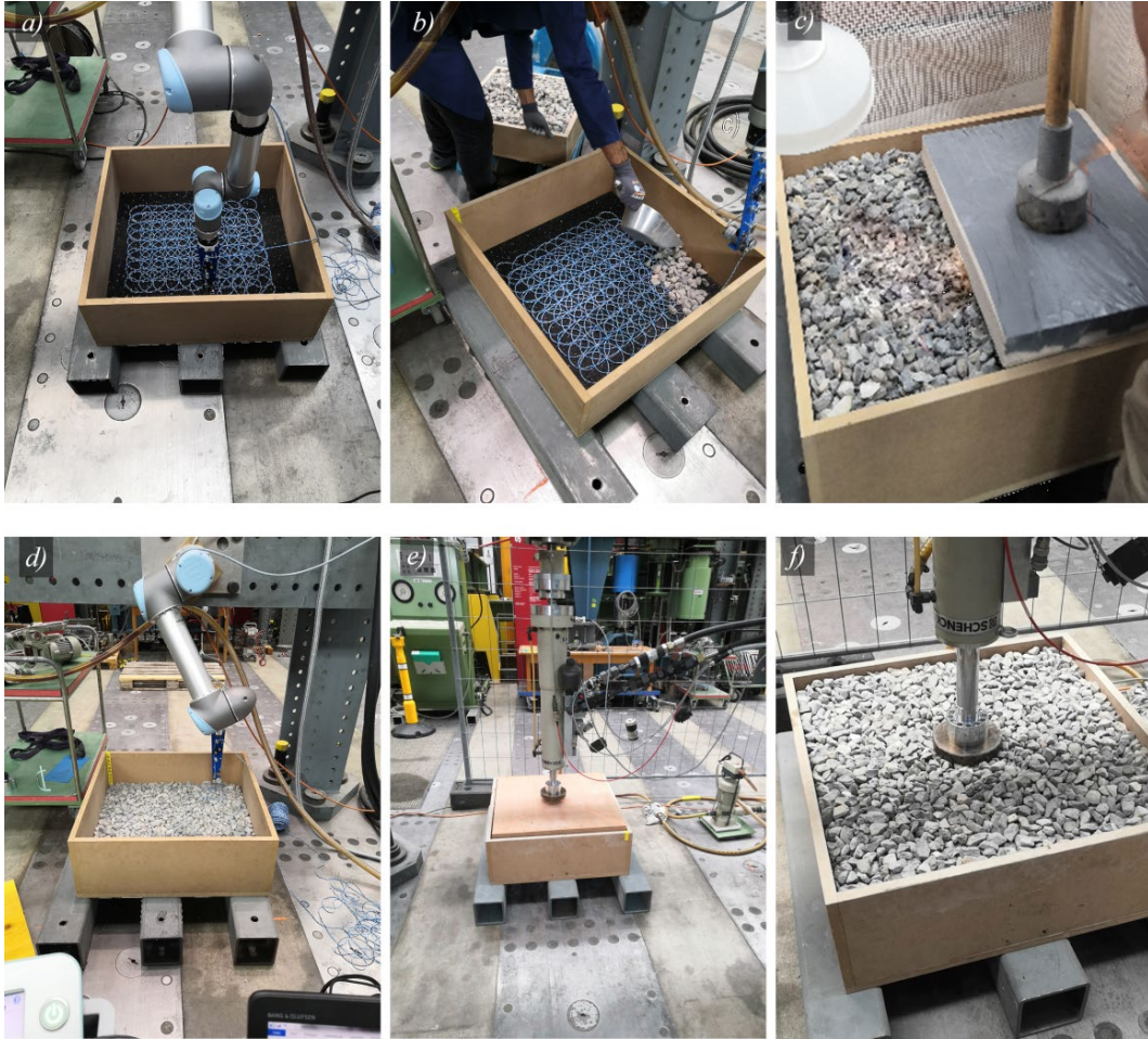
Abb. 10 specimen preparation: a) deployment of the first string reinforcement layer with a robotic arm, b) addition of first aggregate layer, c) densification of individual layers, d) deployment of consecutive reinforcement and aggregate layers e) final compaction and d) cycling loading setup.
