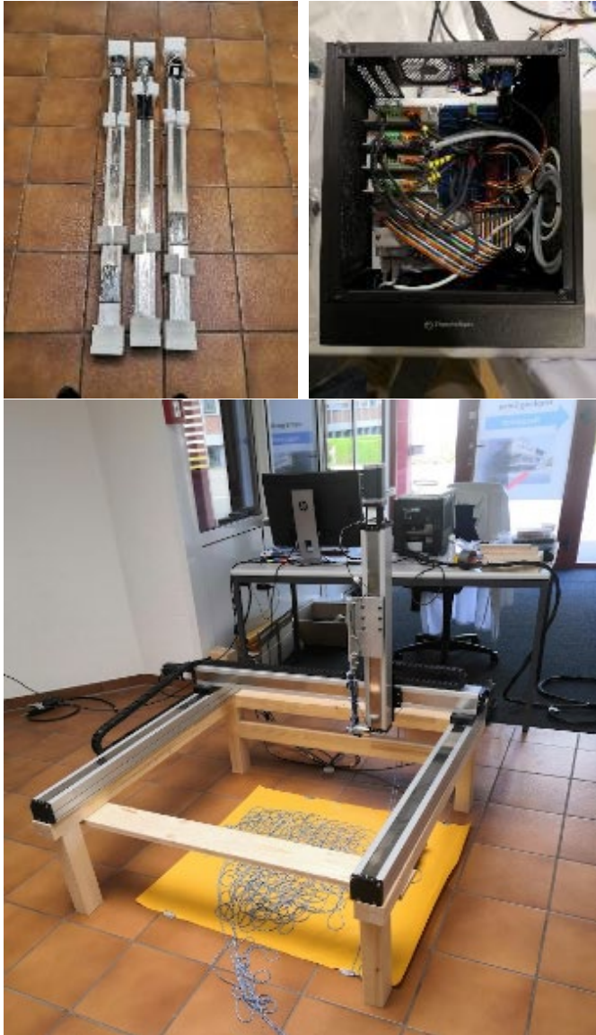
Abb. 14 view of the beams used to build a self-made Cartesian 3D printer, including the electronics and final setup.
