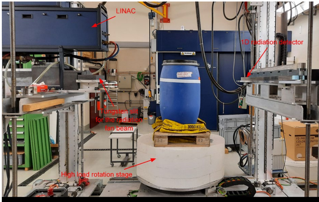
Abb. 34 photograph of the very-high energy X-ray tomograph at Empa's Center for X-ray Analytics, with details of the setup evidenced.
