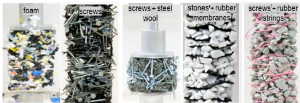
Abb. 2 compression tests of a wide range of jammed material systems and reinforcements (from [13]).
