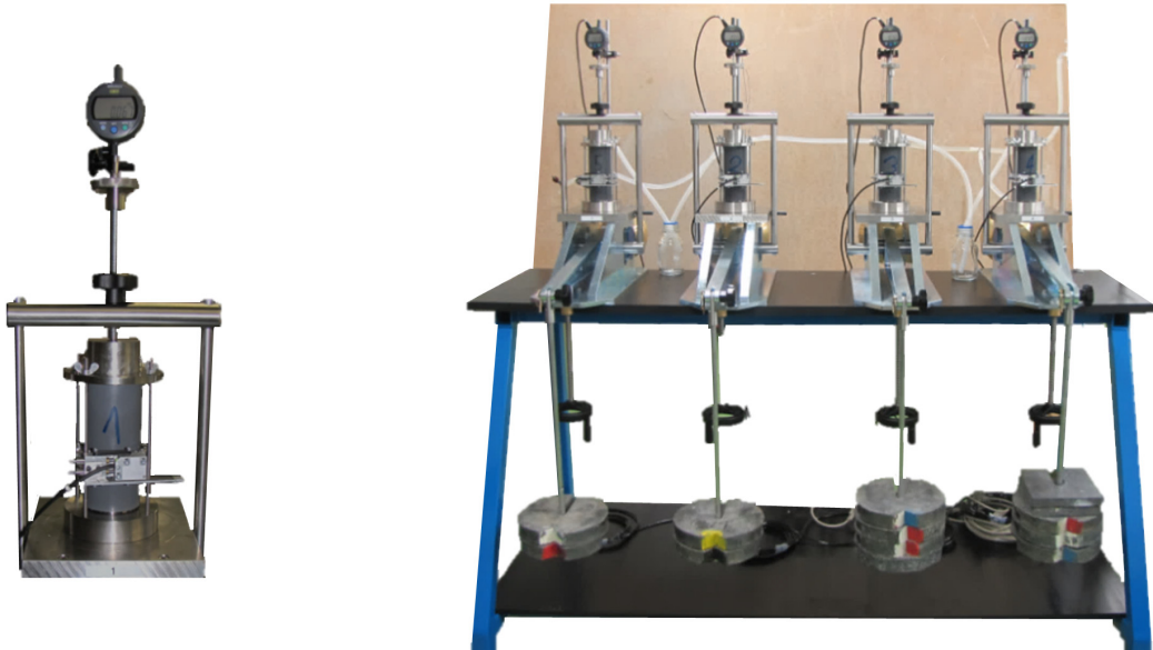
Figure 12.35 Apparatus for flexible oedometer tests.
