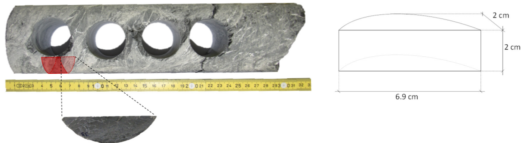
Figure 13.2 Left: Bore core Belchen BH3 3.1-3.4m and example for one segmental sample. Right: typical dimensions of segmental samples.
