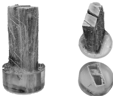
Figure 11.4 Photographs of the sample BB 1f after embedding in epoxy (left) and after sawing (right).
