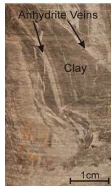
Figure 3.9 Typical rock fabric of the test specimens
